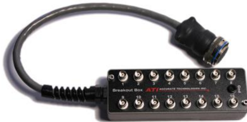
Figure 72: ATI EDAQ to capture ion signals [35]
